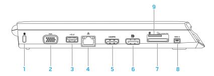
Security cable slot — Attaches a commercially available security cable to the computer.
